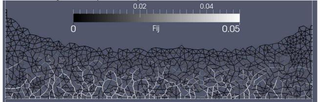
Figure 4: 2D simulation of transient clogging of a filter. Network of contact forces between particles.
