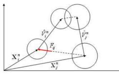
**Figure 2**: Particles initial position, directional vector, and a priori velocities and particles final positions given  $\mathbf{F}_{ij} = 0$ Subtracting equations of motion for particles i and j in (9) give the following relation:
