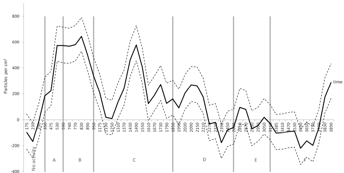
Figure 6. Number concentration of particles emitted at the source after the procedure of removal of the aerosol background as median value with 95%-confidence intervals.
