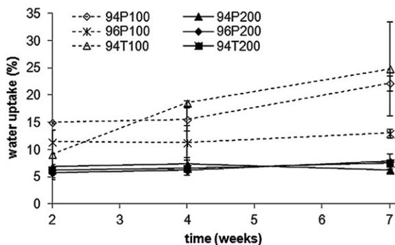
Fig. 2. Water uptake profiles of copolymers during degradation.
