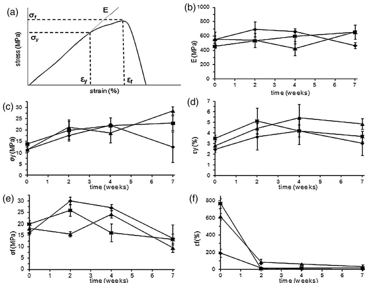
Fig. 6. Evolution of copolymers mechanical properties during degradation. (a) Representation of a typical tensile stress-strain curve obtained for a copolymer. (b) Young's modulus  $E$ . (c) yield stress  $\sigma_y$ . (d) yield strain  $\varepsilon_y$ . (e) Stress at failure  $\sigma_f$ . (f) Strain at  $\varepsilon_f$  failure.
