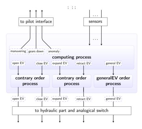
Figure 3: Computing module implementation.
