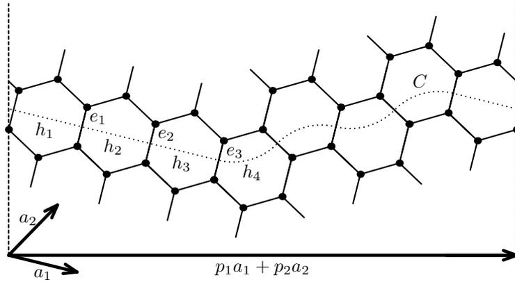
Figure 1: An example of a nanotube of type  $(6, 2)$ .
