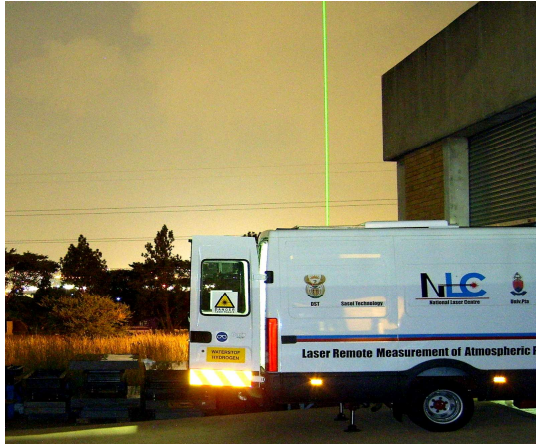
Figure 3: CSIR-NLC-Mobile LIDAR system
