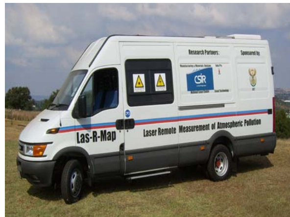
Figure 1. The external view of mobile LIDAR van.
