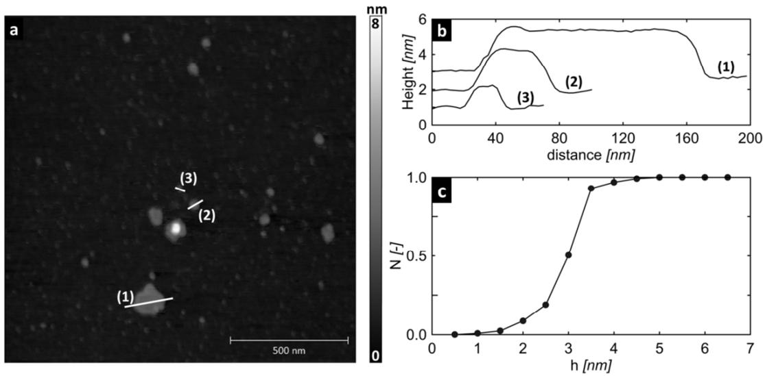
**Figure 1.** Thickness  $h$  of the NMG nanoplatelets. (a) AFM height image, (b) Height profiles of NMG platelets extracted from AFM images (the profiles have been shifted along y-axis for clarity) and (c) Cumulative distribution of the NMG thickness.
