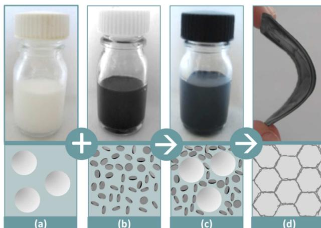
**Figure 4.** Processing steps of the nanocomposite materials, (a) blank latex, (b) NMG suspension, (c) NMG-latex blend, (d) flexible and conductive material obtained after water evaporation and film formation.
