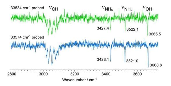
Figure 2: IR-UV hole burning spectra of the two species (isomers or hot bands) probing the band at 33574 cm<sup>-1</sup> (lower panel) and the small band at 33634 cm<sup>-1</sup> (upper panel).
