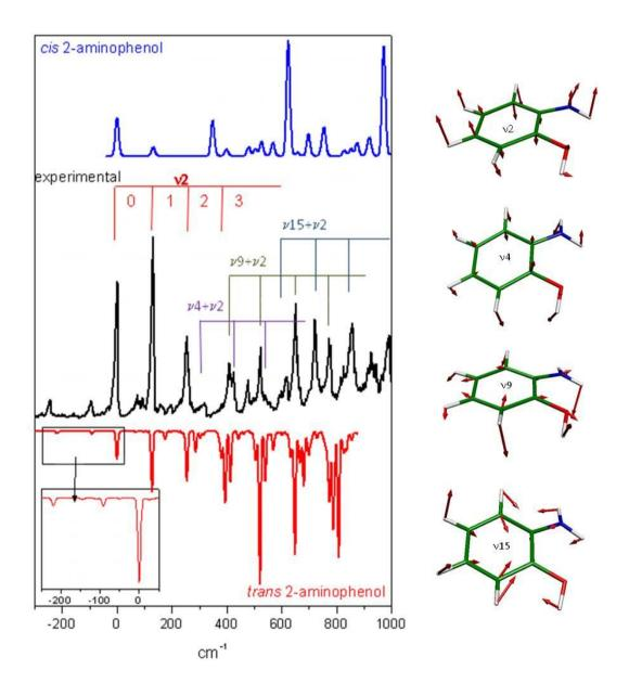
Figure 5: Left panel from top to bottom: simulated spectra using the ground and excited state frequencies calculated at the RI-CC2/aug-cc-pVDZ level for the *cis* isomer (blue) and for the *trans* isomer with a scaling factor of 0.82 (red) and experimental spectrum (black). The assignment of the vibrational bands is also shown on top of the experimental spectrum. Right panel: Scheme of the vibrational modes involved in the spectrum.
