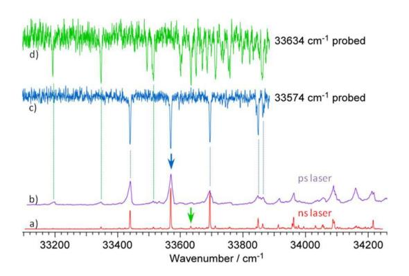
Figure 1: REMPI excitation spectrum recorded with a) ns laser with 0.08 cm<sup>-1</sup> resolution; b) ps lasers with 15 cm<sup>-1</sup> resolution. UV-UV hole burning spectrum pumping the band at c) 33574 cm<sup>-1</sup> (blue arrow) and d) the small band at 33634 cm<sup>-1</sup> (green arrow).
