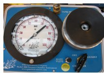
a pressure bomb to assess xylem water potentials ( \Psi_x )
