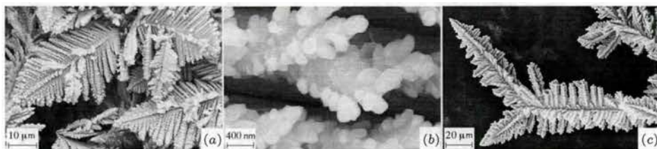
Fig. 3. \text{pH} = 2 , H = 0 , SEM images. (a): typical dendrites; (b): small crystallites on the top of the branches; (c): quite a rare case of a dendrite with 90^\circ angle between the branches, revealing either a fcc structure or a hcp structure with the c -axis within the growth plane.
