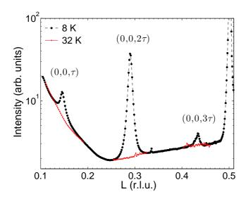
FIG. 2. (Color online) Scan along the [001] direction in reciprocal space at an incident photon energy of 709.8 eV corresponding to the Fe L<sub>3</sub> edge. r.l.u. denotes reciprocal-lattice units. Dashed (black) line represents data collected at 8 K while the continuous (red) line represents data collected above  $T_N$  at 32 K. The peak visible in the vicinity of 0.5 r.l.u. corresponds to higher harmonic contamination from the (001) reflection.
