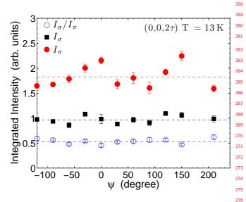
FIG. 5. (Color online) Azimuthal angle dependence of the  $(0,_{277}, 0, 2\tau)$  superstructural reflection. The line represents a fit to  $_{278}$  the data with a constant ( $\chi^2 = 1.6$  for the ratio  $I_{\sigma}/I_{\pi}$ ), as  $_{279}$  expected form the model presented in the text. Measurements were performed in the vicinity of the Fe L<sub>3</sub> edge (E=709.8 eV). The azimuthal angle equals zero when the [100] direction is<sup>281</sup> in the scattering plane.
