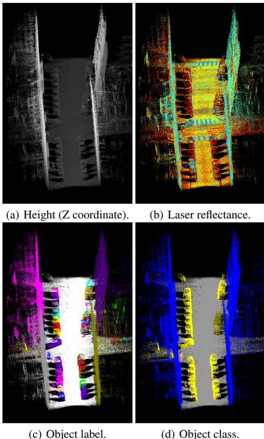
Figure 2: “GT\_Madame1.2.ply” file: 3D point cloud colored by its available fields. For the object *label*, each color represents a different object (only for visualization purposes, some colors have been repeated). For object *class* visualization: facades (blue), ground (gray), cars (yellow), motorcycles (olive), traffic signs (goldenrod), pedestrians (pink).
