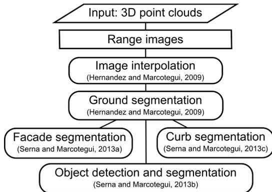
Figure 4: Work-flow of our automatic segmentation methodology.
