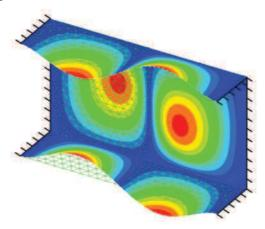
As the precision of the calculated frequencies has to be better than 1%, hammer impact tests were conducted in order to adjust the finite element model to the real behaviour of the part. These tests were made before and after the machining. The damping ratio was obtained by hammer test because it is impossible to predict accurately.
