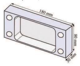
This part is made of two distinct types of thin walls: the floor and the lateral wall. The workpiece is made of an aluminium alloy 7075T6 like structural parts. The dimensions are chosen in order to correlate with an industrial part. The thicknesses of the walls after machining are respectively of 1 mm for the floor and 3 mm for the walls.
