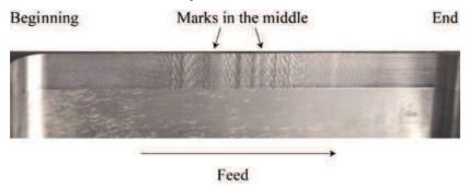
Regarding the walls, Figure 11 shows the machined thin wall with the cutting conditions mentioned above. The machining was unstable for a depth of cut of 5 mm, in fact, the marks appear only in the middle of the wall, where the apparent stiffness is lower (see Figure 11). On the other hand, the test with a depth of cut of 3 mm was stable, with a good surface roughness without any marks. It can be concluded that the real limiting depth of cut was lower than the one calculated with the lobes.
