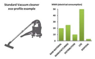
Figure 4. Example of standard vacuum cleaner eco-profile [25]
