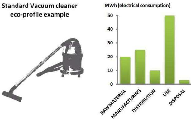
Figure 4. Example of standard vacuum cleaner eco-profile [25]
