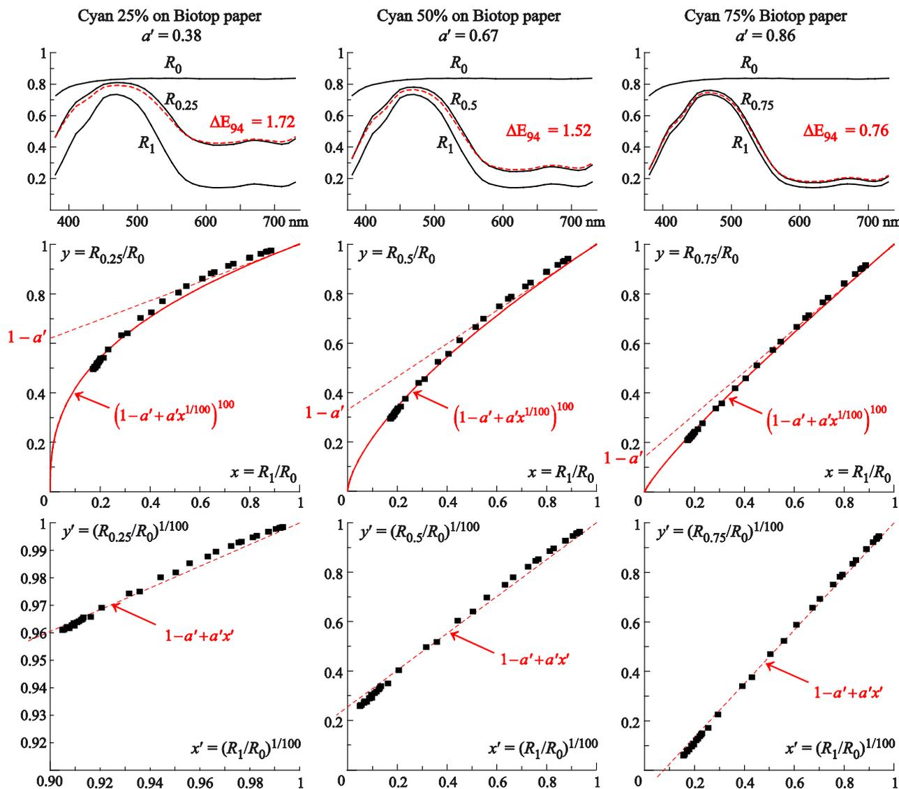
Figure 7. Similar graphs as in Figure 6 for cyan ink halftones printed at 0.25, 0.5 and 0.75 nominal surface coverages on Biotop non-calendered paper. The Yule-Nielsen functions were calculated with  $n = 100$ .
