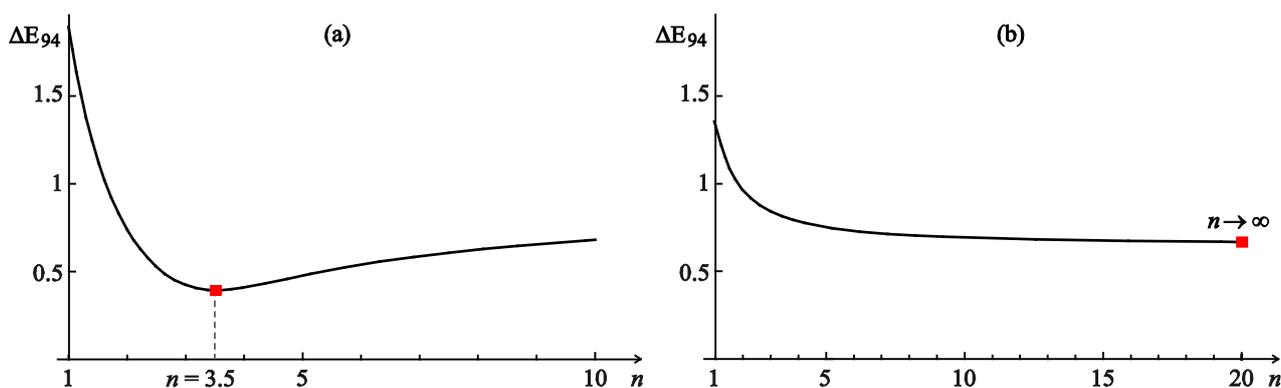
Figure 4. Variation as a function of the  $n$  value of the average  $\Delta E_{94}$  computed from the predicted and measured spectral reflectances of the 36 single-ink halftones displayed in Figure 2, in the case of (a) inkjet CMY colors printed at 150 lpi on glossy coated paper and (b) in the case of CMY colors printed at 100 lpi on common office paper.
