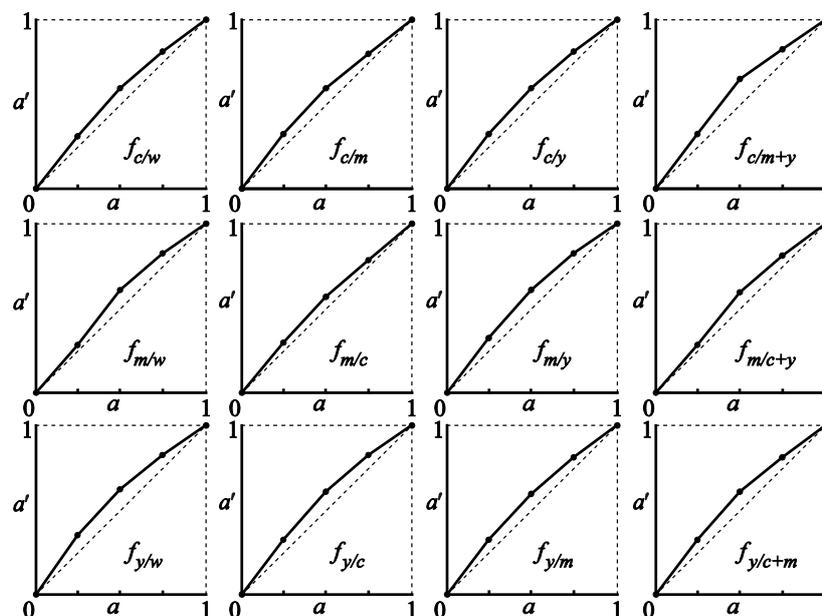
Figure 3. Example of ink spreading functions giving the effective surface coverage  $a'$  of each ink superposed with each colorant made of the other two inks at the surface coverages 1 or 0, as functions of the nominal surface coverage  $a$ .
