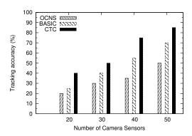
Fig. 2. Tracking accuracy vs. number of Camera Sensors
