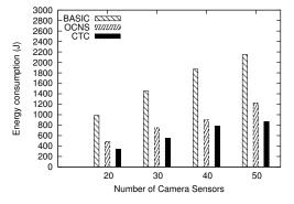
Fig. 3. Energy Consumption vs. number of Camera Sensors
