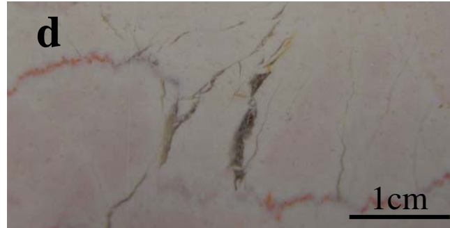
Fig 9: Zoom-in on the slab of Fig 4 showing small-scale field-relations between fractures and stylolites and between the stylolites themselves.
