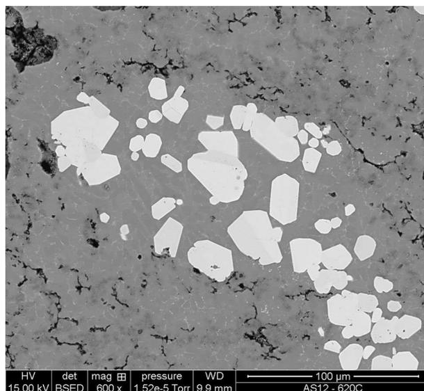
**Fig. 1** Backscattered micrograph of an Al-12 at.%Si liquid saturated in Ti after 140 h at 620 °C and water quenching, revealing the presence of crystals
