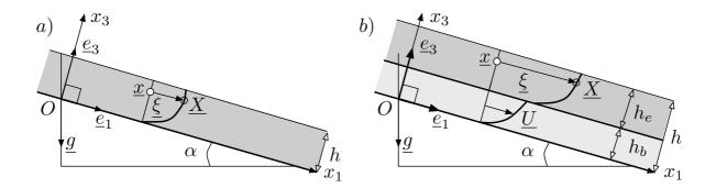
Figure 1. a) Layer of elastic solid on a tilted plane. b) Layer of Bingham fluid for  $0 \le x_3 \le h_b$  under a layer of solid for  $h_b \le x_3 \le h$ .
