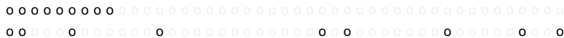
Figure 2.: On top is the output pupil of a fully redundant configuration. On the bottom is the non-redundant configuration used in the prototype FIRST instrument.
