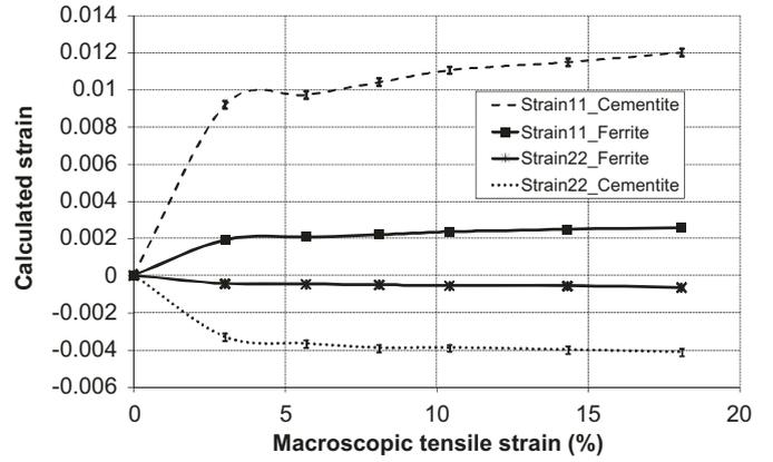
**Fig. 7.** Evolution of elastic strains  $\epsilon_{11}^e$  and  $\epsilon_{22}^e$  for both ferrite and cementite phases during loading: synchrotron measurements. The error bars for elastic strain uncertainties are provided (see text for values).
