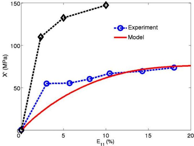
**Fig. 13.** Bauschinger stress  $X'$  model predictions (bold line) by using ILMF reference stress curves of Fig. 10, and experimental estimations (circles) by using both phase stresses of Fig. 8. The experimental Bauschinger stress  $X$  reported in Fig. 4 and derived from the macroscopic data in Fig. 3 is also reported (diamonds).
