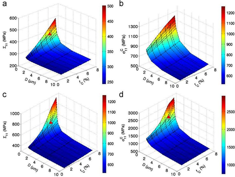
**Fig. 12.** ILMF model predictions with materials parameters given in Table 2 of macroscopic tensile stresses  $\Sigma_{11}$  at 5% of strain (a), 20% of strain (c) and particle tensile stresses  $\sigma_{11}^c$  at 5% of strain (b), 20% of strain (d). The values are reported as functions of  $f_c$  (particle volume fraction) and  $D$  (equivalent average particle size diameter). The triangles indicate the predicted values for the ferrite-cementite steel studied in the present paper.
