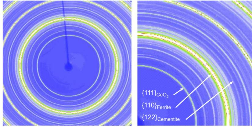
**Fig. A2.** Ring diffraction pattern with different rings corresponding to the two phases of the material analyzed and the CeO<sub>2</sub> calibrant.
