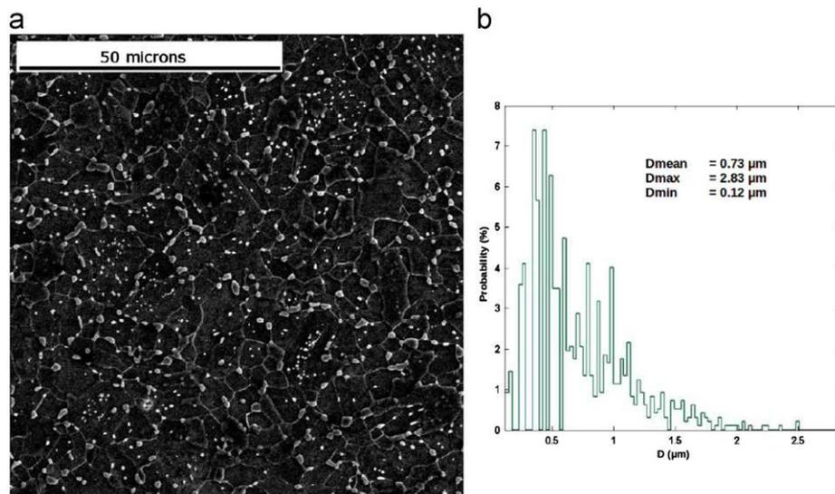
Fig. 1. (a) SEM image of the designed ferrite- $\text{Fe}_3\text{C}$  carbides steel with particle spatial distribution, (b) probability distribution of measured particle size  $D$ .
