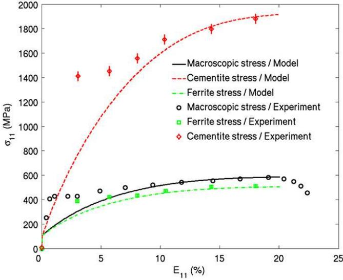
**Fig. 10.** Macroscopic and phase stresses predicted by the model with an aspect ratio of 1.5 for ellipsoidal particles aligned in the tensile direction. Experimental estimations of Fig. 8 are superimposed for comparison.
