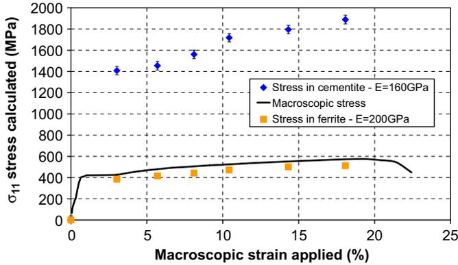
**Fig. 8.** Evolution of the  $\sigma_{11}$  stress for both ferrite and cementite phases during loading.  $E_{(110)}^{Fe_s} = 200 \pm 1$  GPa and  $E_{(122)}^{Fe_sC} = 160 \pm 3$  GPa. The error bars for stress uncertainties in cementite are provided (see text for values).
