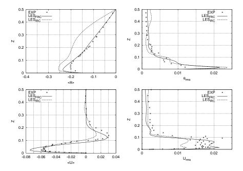
Fig. 13. Vertical profiles along the centerline  $(x,y) = (A_x/2, A_y/2)$  of the time-averaged temperature  $(<\theta>)$ , the horizontal velocity (<U>) and their respective rms fluctuations (left). Comparison between FRC results and experimental data.
