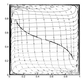
Fig. 11. Superimposition of the isocontours of temperature  $\langle \theta \rangle$  and streamlines in the time-averaged flow on the vertical plane close to the front wall (y = 0.00866) for the FRC cavity.
