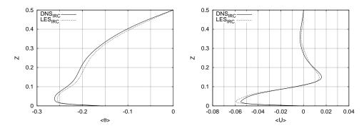
Fig. 3. Vertical profiles of the time-averaged temperature ( $<\theta>$ ) and the horizontal velocity (<U>) along the vertical centerline  $(x,y)=(A_x/2,y=A_y/2)$  in the IRC case. Comparison between DNS and LES.
