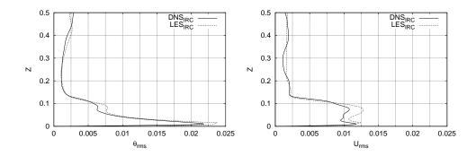
Fig. 5. Vertical profiles of the rms fluctuations of temperature  $(\theta_{rms})$  and vertical velocity  $(U_{rms})$  along the vertical centerline  $(x,y)=(A_x/2,y=A_y/2)$  in the IRC case. Comparison between DNS and LES.
