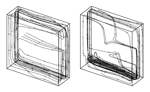
Fig. 8. Streamlines in the time-averaged flow for IRC (left) and FRC (right).
