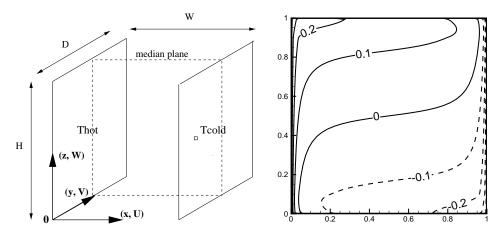
Fig. 1. Geometry definition (left) and smoothed front and rear walls temperature distributions reconstructed from infrared camera measurements (Salat, 2004) (right).
