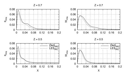
Fig. 4. Horizontal profiles of the rms fluctuations of temperature  $(\theta_{rms})$  and vertical velocity  $(W_{rms})$  at  $y = A_y/2$  and two different heights in the IRC case. Comparison between DNS and LES.
