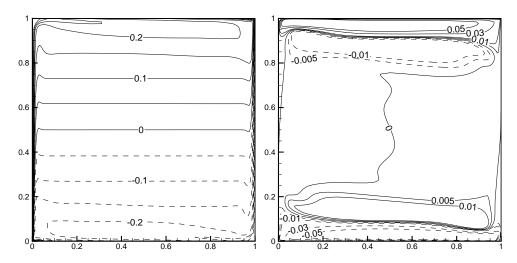
Fig. 9. Isocontours of temperature  $<\theta>$  (left) and horizontal velocity < U> (right) in the vertical mid-depth plane  $(y=A_y/2)$  in the FRC.
