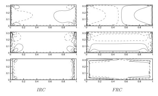
Fig. 10. Isocontours of velocity components the horizonin tal mid-height plane (z $A_z/2$ ). From top to bottom, hor-=>= [ $\pm 0.0002; \pm 0.002$ ]), spanwise velocizontal velocity (< >= $[\pm 0.0002; \pm 0.001; \pm 0.002]$ ) and vertical velocity  $(<W>=[\pm 0.0002;\pm 0.002])$ . Comparison between IRC (left) and FRC (right).
