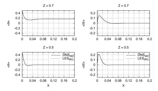
Fig. 2. Horizontal profiles of the time-averaged temperature ( $<\theta>$ ) and vertical velocity (<W>) at  $y=A_y/2$  and two different heights in the IRC case. Comparison between DNS and LES.
