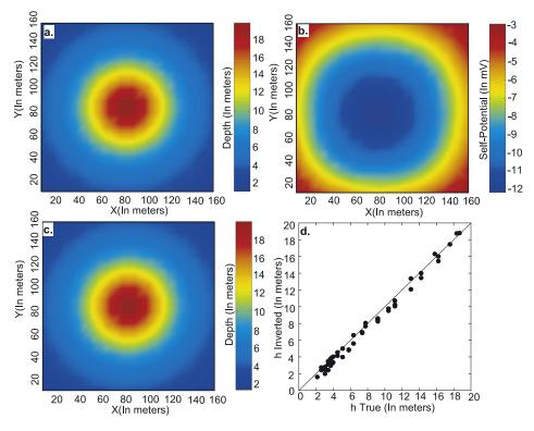
**Figure 2.** Synthetic test. (a) Synthetic case showing a Gaussian depression of the water table. (b) Distribution of the resulting self-potentials at the ground surface (with c' = -4 mV/m and  $h_0 = 2$  m). (c) Inverted result of the water table (RMS error 1.15%). (d) True depth of the water table versus the inverted depth of the water table.
