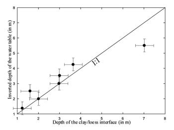
**Figure 6.** Inverted depth of the loess/clay-with-flint interface versus the height of the interface determined from the electrical resistivity data (r = 0.88). The error associated with the deepest point is coming from the small density of measurements performed over the sinkholes in the present study.
