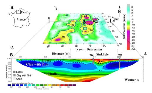
**Figure 3.** (a) Location of the test site in Normandy (France). (b) Self-potential map in Spring 2005. The anomalies A1 and A2 are sinkholes while A3, B2, and B3 are crypto-sinkholes. Ref represents the reference of the self-potential data and P1 is the resistivity profile. (c) Electrical resistivity tomogram inverted with RES2DINV [*Loke and Barker*, 1996] (Wenner- $\alpha$  array, electrode spacing 3 m, iteration 4, RMS error 1.4%).
