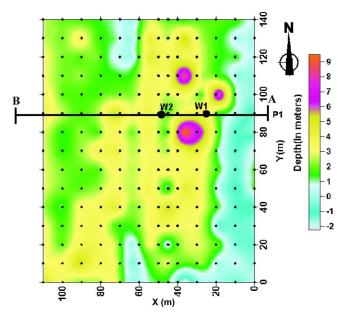
**Figure 4.** Inversion of the interface between the loess and the clay-with-flint formations. (RMS error 6.12%). The inversion shows clearly a wide depression of the interface with a North-South trend along which the sinkholes are aligned. The circular depressions of the water table correspond to the sinkholes.
