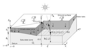
**Figure 1.** Sketch of the geometry of the water table corresponding to interface between an unconfined shallow aquifer (volume  $\Omega_i$ ) and the unsaturated (vadose) zone (volume  $\Omega_e$ ).
