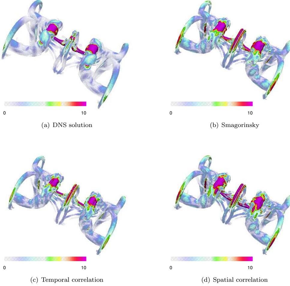
Figure 6. Iso-surfaces of  $Q$  magnitude for the dimensionless time  $t = 15$ : (a)  $256^3$  grid points DNS solution, (b) Smagorinsky solution onto  $128^3$  grid points, (c) solution computed with temporal covariance on  $128^3$  grid points and (d) solution computed with spatial covariance on  $128^3$  grid points.
