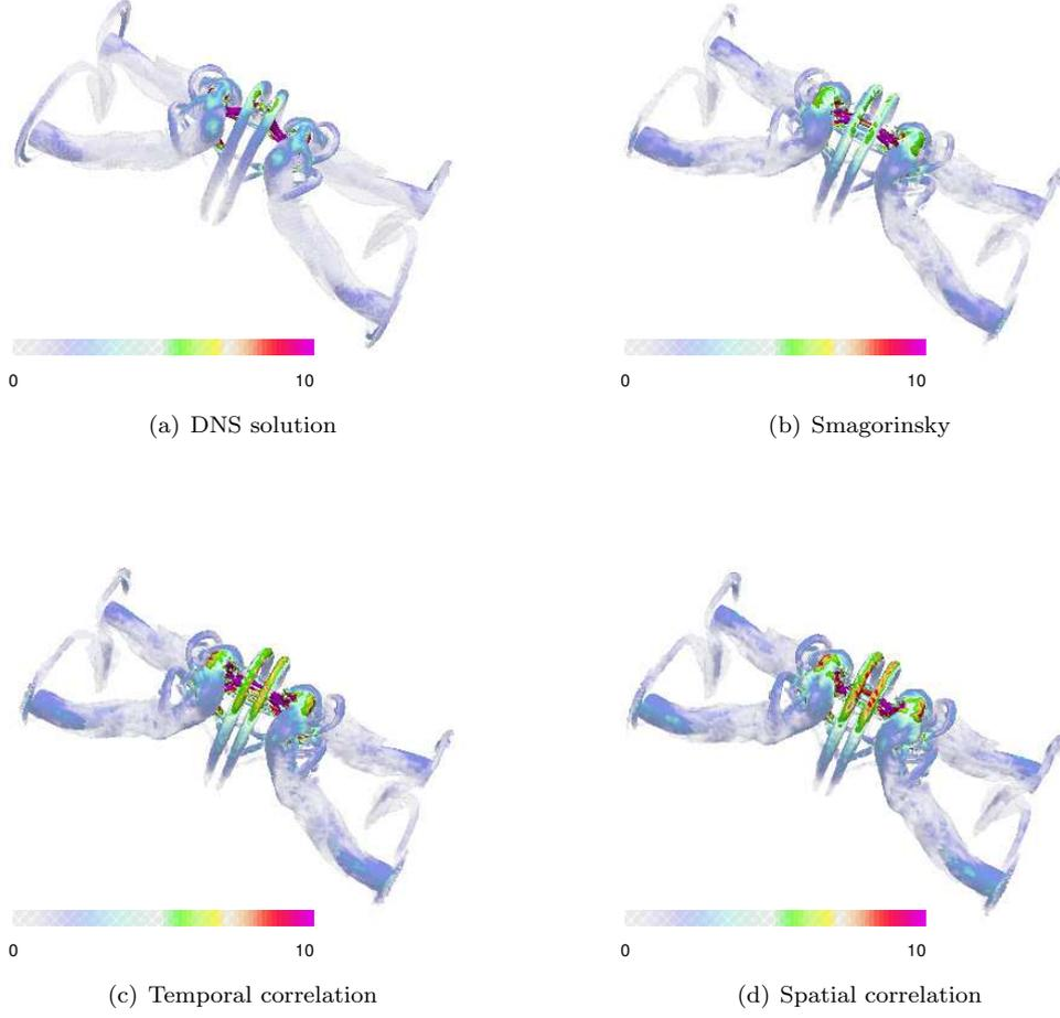
Figure 5. Iso-surfaces of  $Q$  magnitude for the dimensionless time  $t \approx 10$ : (a)  $256^3$  grid points DNS solution, (b) Smagorinsky solution onto  $128^3$  grid points, (c) solution computed with temporal covariance on  $128^3$  grid points and (d) solution computed with spatial covariance on  $128^3$  grid points.
