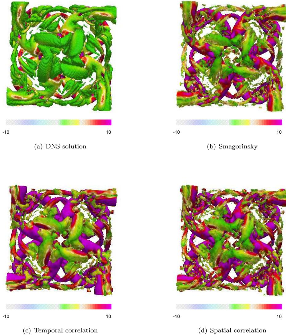
Figure 3. Iso-surfaces  $Q = 1$  for the dimensionless time  $t \approx 9$ : (a)  $256^3$  grid points DNS solution, (b) Smagorinsky solution onto  $128^3$  grid points, (c) solution computed with temporal covariance on  $128^3$  grid points and (d) solution computed with spatial covariance on  $128^3$  grid points.
