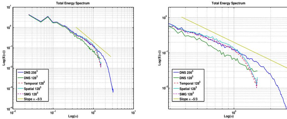
Figure 2. Different solutions total energy spectrums (left) and zoom in at the tail (right), for the dimensionless time  $t \approx 9$ .
