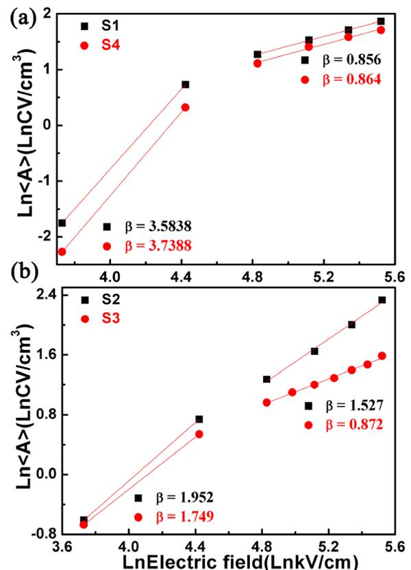
FIG. 4. The hysteresis area  $\langle A \rangle$  as a function of electric field  $E$  of the films with (a) Pt and (b) LNO as top electrodes.
