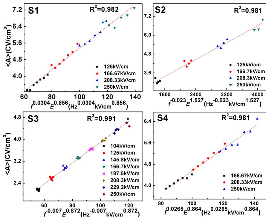
FIG. 5. Scaling plots of hysteresis area  $\langle A \rangle$  against  $E$  and  $f$  for the PZT thin films with different interface configurations.
