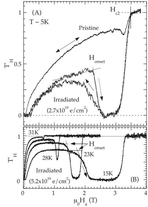
FIG. 1. (a) Field dependence of the ac transmittivity in a pristine, and in an irradiated  $\text{MgB}_2$  single crystal ( $2.7 \times 10^{19} e^- \text{cm}^{-2}$ ). Note the hysteresis between increasing and decreasing field branches for  $H_a \sim H_{\text{onset}}$  after irradiation. (b) Transmittivity of a crystal irradiated to  $5.2 \times 10^{19} e^- \text{cm}^{-2}$ , at the indicated temperatures (ascending field branch only).
