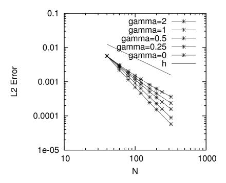
Figure 6: The error is plotted in log scale versus the number of cells per direction in the academic square. Each curve corresponds to a value of  $\gamma \in \{0, \frac{1}{4}, \frac{1}{2}, 1, 2\}$ , plus a reference line for order one. One sees that the order of convergence is an increasing function of  $\gamma$ .
