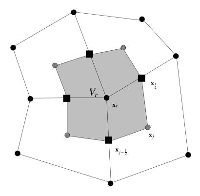
Figure 5: Definition of the control volume  $V_r$  around vertex  $\mathbf{x}_r$ . The control volume around the vertex  $\mathbf{x}_r$  is defined by the closed loop that joins the center of the cells  $(\mathbf{x}_j)$ 's and the middle of the edges  $(\mathbf{x}_{j+\frac{1}{2}})$ 's).
