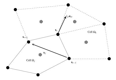
Figure 4: Notation for node formulation. The corner length  $l_{jr}$  and the corner normal  $\mathbf{n}_{jr}$  are defined in equation (41). The point  $\mathbf{x}_j$  is an arbitrary point inside the cell, typically the centroid of the cell or an averaged of the corners.
