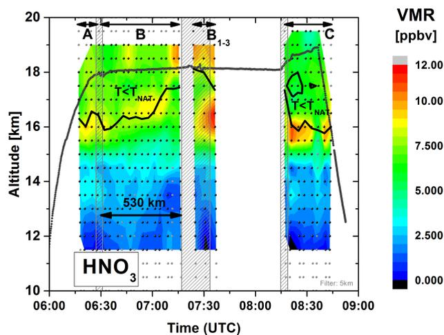
**Figure 6.** Vertical cross section of gas-phase  $\text{HNO}_3$  retrieved from the MIPAS-STR observations associated with the flight on 25 January 2010. Other parameters as in Fig. 4 (from Woiwode PhD thesis, 2013, with modifications).
