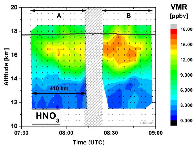
**Figure 10.** Vertical cross section of gas-phase  $\text{HNO}_3$  retrieved from the MIPAS-STR observations associated with the flight on 30 January 2010. Compare Fig. 6 (from Woiwode PhD thesis, 2013, with modifications).
