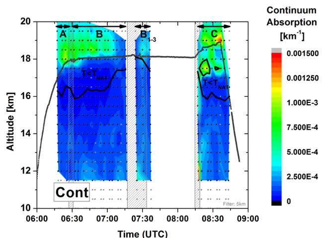
**Figure 5.** Vertical cross section of continuum absorption retrieved from the MIPAS-STR observations associated with the flight on 25 January 2010. Enhanced continuum absorption indicates cloud/aerosol particles. Other parameters as in Fig. 4 (from Woiwode PhD thesis, 2013, with modifications).
