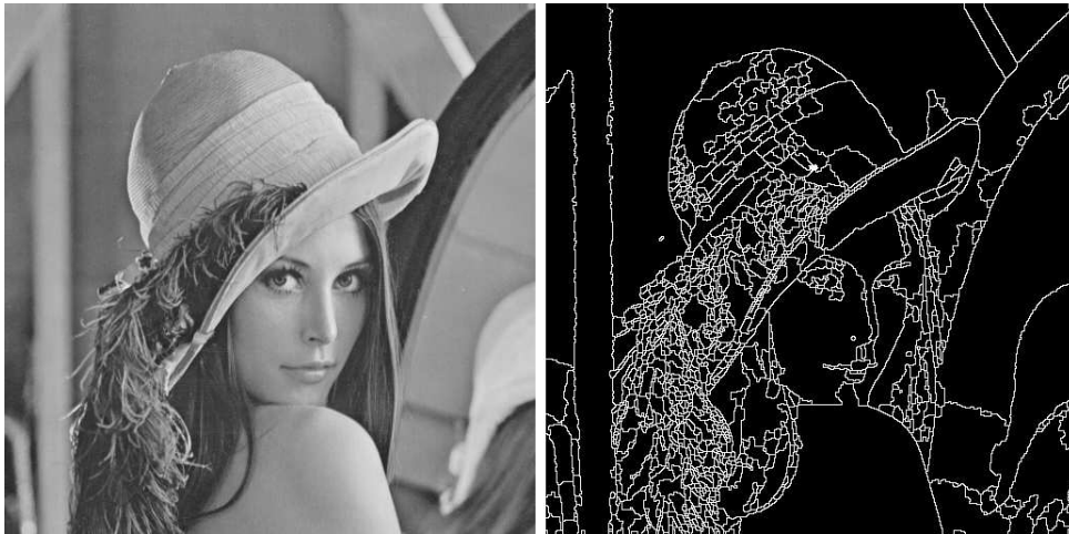
Figure 4: Image of Lena (left), watershed computed on gradient and hmin of the image (right)
