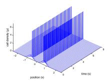
Figure 6: Wrong velocity discretization for (1.1)
