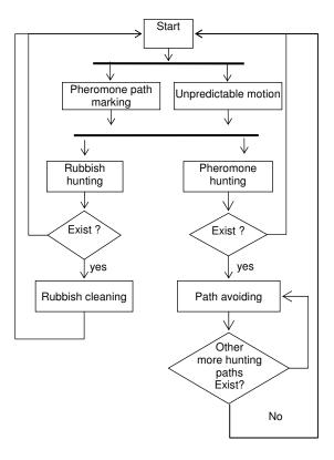
Figure 1. Collaborative cleaning task based on Counter-Ant Algorithm.
