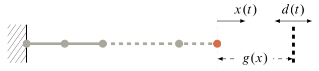
Figure 4. Simplified rod model: contact (●) and internal nodes (●)
