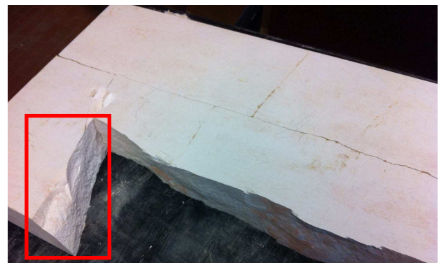
Fig. 9. Fractured block. The fracture in correspondence to the hole 7 is shown in the lower left side.
