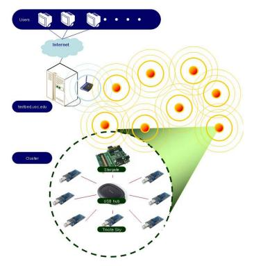
Fig. 14 Tutornet: 3-tiered WSN testbed.
