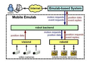
Fig. 15 The software architecture of Mobile Emulab [108].
