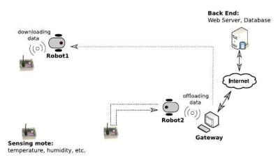
Fig. 18 Overall system architecture: synergy between mobile robots and WSN[128].
