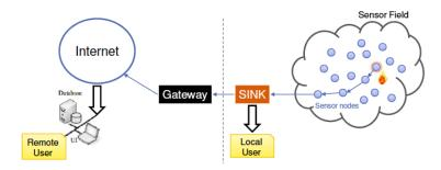
Fig. 2 Wireless Sensor Network (WSN) [42].
