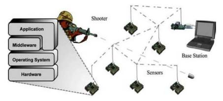
Fig. 9 System architecture in the counter-sniper application PinPtr[72].
