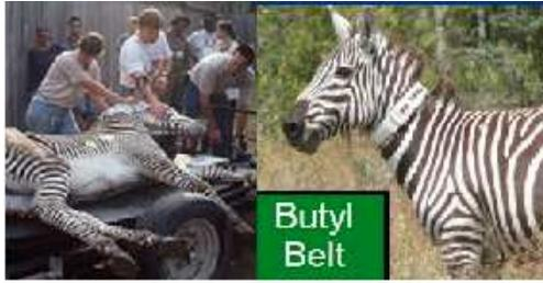
Fig. 10 The ZebraNet sensor collar, attached to a Zebra [74].
