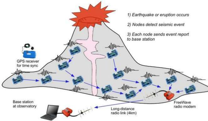
Fig. 11 Volcan Reventador deployment for volcano monitoring [76].
