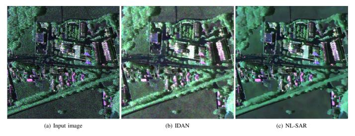
Fig. 16. Restoration of a polarimetric F-SAR image near Kaufbeuren (Germany) ©DLR: (a) original image; b) speckle reduction with IDAN; (c) speckle reduction with NL-SAR.
