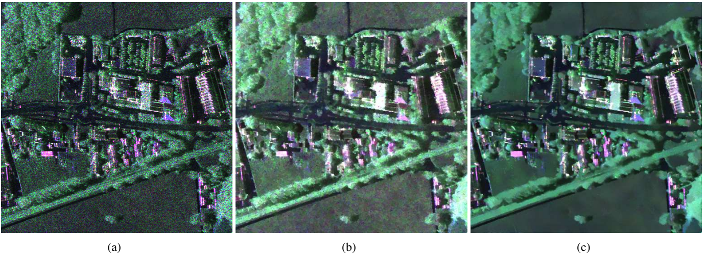
Fig. 16. Restoration of a polarimetric F-SAR image near Kaufbeuren (Germany) ©DLR: (a) original image; (b) speckle reduction with IDAN; (c) speckle reduction with NL-SAR.
