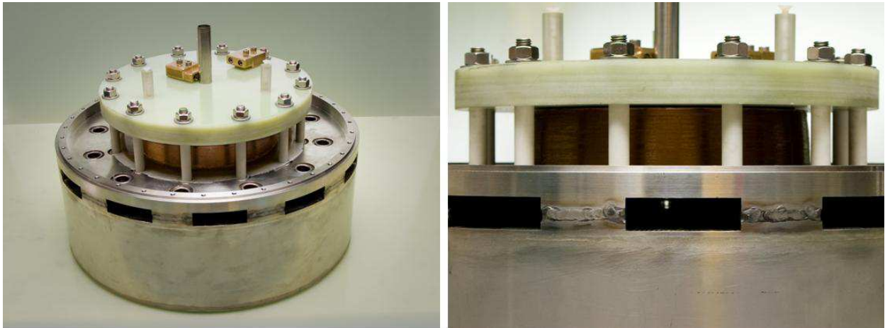
FIG. 2. (Color online) Pictures of the split-pair magnet mounting. Only the upper coil is visible, the lower coil being integrated into the lower part of the liquid nitrogen bath.
