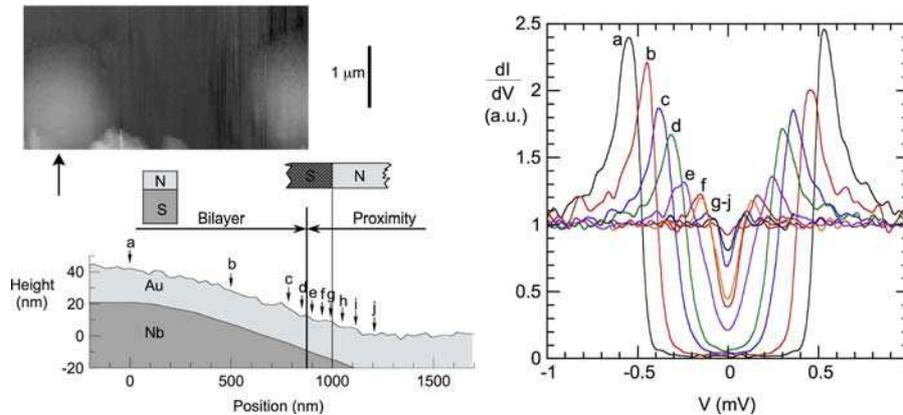
We have carried out a similar study in Nb/Au bilayers with an increased gap thanks to a larger thickness of the Nb layer [17]. This increased  $\Delta/k_B T$  enabled us to unveil an anomalous behaviour of the local density of states at the surface: a non-zero density of states appears within the mini-gap and increases when the thickness of the Au layer is increased. This behaviour is presumably related to the shape of the Au Fermi surface.
