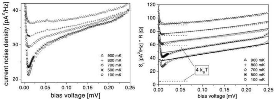
For small voltages ( $V < 50 \mu\text{V}$ ) the experimental data show a nonlinear regime which extends down to its minimum at the Thouless energy. The simple model
