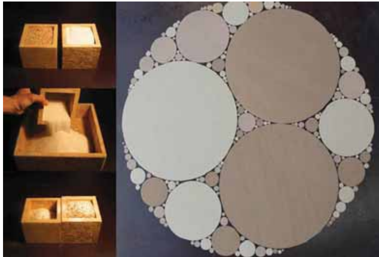
Fig. 4 - Packing experiments and mathematical model of Apollonian packing (© CRAterre-ENSAG)
