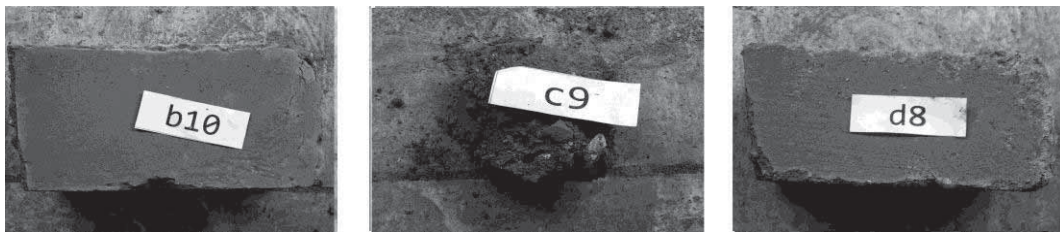
Fig. 1 - Comparison between mixtures with gypsum powder and mixtures without any additive after 6 cycles of immersion. The specimen marked with the letter 'b' contains 15% gypsum powder, the one marked with 'd' contains 25% gypsum powder, while 'c' does not contain any additives.
