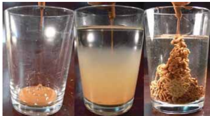
Fig. 2 - Salt concentration in water changes clay mud viscosity because of electrical interactions between clay particles (© CRAterre-ENSAG)
