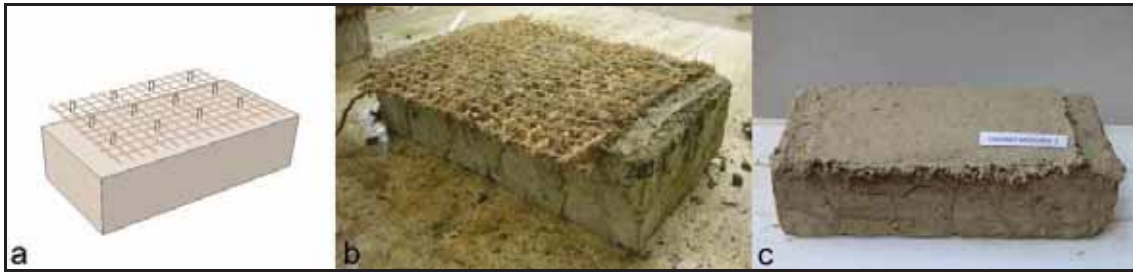
Fig. 1 - Production process of a sample: a) the mesh nailed to the surface. b) the plate plastered. c) COCO_Anchored1
