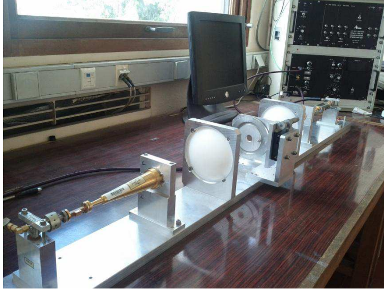
Figure 4. Characterization measurement setup composed of an AB Millimeter VNA and lens-horns antennas [14]
