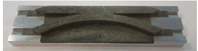
Fig. 13. Dielectric coupler at 30 GHz before being pressed
