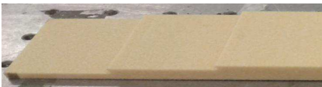
Fig. 6. Stepped sample before being pressed (5, 10, 15mm).
