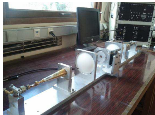
Fig. 8. Photograph of the free space measurement setup composed of horn-lens antennas and support of sample under test.
