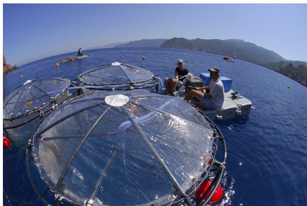
Fig. 7. Sampling the mesocosms. Each cluster of three mesocosms is simultaneously sampled a plastic platform by a team of two scientists. Overall a sampling sequence duration was less than two hours (photo: D. Luquet OOV).
