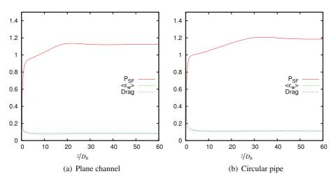
**Fig. 8.** Evolutions of sub-filter production, drag and wake dissipation for turbulent plane channel flows. Each quantity  $\xi$  is adimensioned by  $|\xi_{inlet} - \xi_{\infty}|$ . The length of establishment associated to  $P_{SF}$  is much larger than the one of the drag and wake dissipation.
