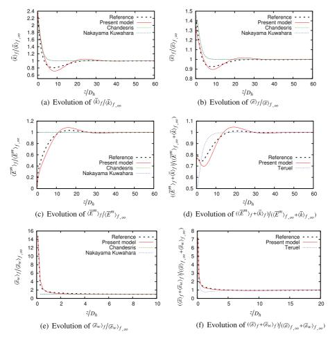
**Fig. 9.** Macroscopic turbulence model results for turbulent flow in stratified porous media composed of flat plates,  $Re = 7.6 \times 10^4$ ;  $\langle \bar{k}_0 \rangle_f / \langle \bar{k}_1 \rangle_{f,\infty} = 4$ . Comparison of the present model to reference results and to the models of Chandesris et al. [1], Nakayama and Kuwahara [13] and Teruel and Rizwan-uddin [22].
