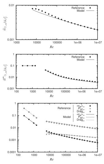
Fig. 6. Asymptotic states: evaluation of expressions (37), (40), (38) and (45) for flows in plane channels. The source terms  $\langle \bar{\epsilon}_w \rangle_{f,\infty}$ ,  $P_{SF\infty}$  and  $\langle \bar{u}_z \rangle_f \overline{F}_{\phi_z}^{\infty}$  are adimensioned by  $\langle \bar{u}_z \rangle_f^3 / 2D_h$ .
