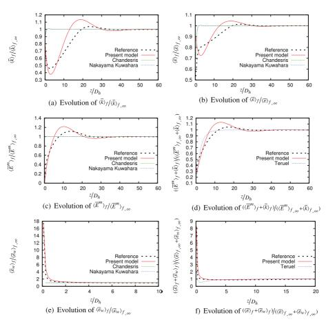
**Fig. 11.** Macroscopic turbulence model results for turbulent flow in stratified porous media composed of flat plates,  $Re = 7.6 \times 10^4$ ;  $\langle \bar{k}_0 \rangle_f / \langle \bar{k} \rangle_{f,\infty} = 0.8$ . Comparison of the present model to reference results and to the models of Chandesris et al. [1], Nakayama and Kuwahara[13] and Teruel and Rizwan-uddin [22].
