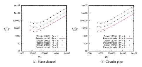
Fig. 4. Comparison between the present model and the model of Drouin et al. [5] for fully developed turbulent flows in pipes.
