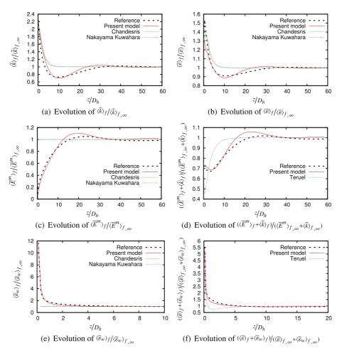
**Fig. 10.** Macroscopic turbulence model results for turbulent flow in stratified porous media composed of circular pipes,  $Re = 7.6 \times 10^4$ ;  $\langle \bar{k}_0 \rangle_{f/\langle \bar{k} \rangle_{f,\infty}} = 4$ . Comparison of the present model to reference results and to the models of Chandesris et al. [1], Nakayama and Kuwahara[13] and Teruel and Rizwan-uddin [22].
