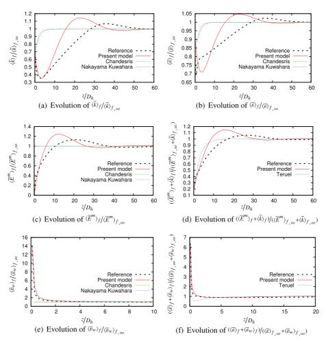
**Fig. 12.** Macroscopic turbulence model results for turbulent flow in stratified porous media composed of circular pipes,  $Re = 7.6 \times 10^4$ ;  $\langle \bar{k}_0 \rangle_f / \langle \bar{k} \rangle_{f,\infty} = 0.8$ . Comparison of the present model to reference results and to the models of Chandesris et al. [1], Nakayama and Kuwahara[13] and [22].
