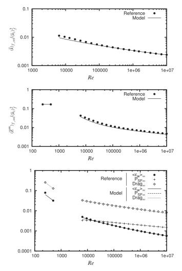
Fig. 7. Asymptotic states: evaluation of expressions (37), (40), (38) and (45) for flows in circular pipes. The source terms  $\langle \bar{e}_w \rangle_{f,\infty}$ ,  $P_{SF\infty}$  and  $\langle \bar{u}_z \rangle_f \overline{F}_{\phi_z}^{\infty}$  are adimensioned by  $\langle \bar{u}_z \rangle_f^3 / 2D_h$ .
