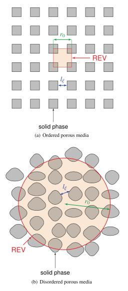
Fig. 2. Representative Elementary Volume in ordered and disordered porous media.
