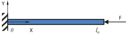
Fig. 5. Cantilever inflatable beam.
