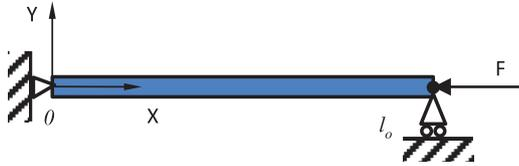
Fig. 6. Simply supported inflatable beam.
