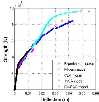
Figure 8: Calibration results of the different models (pushover loading)
