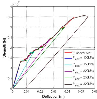
Figure 12: Influence of  $P_{max}$  on the structure response
