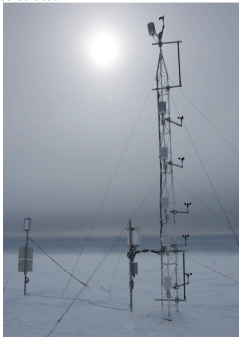
Figure 3. The D17 7 m-mast Automatic Weather and Snow Station in February 2010 with the two one-meter second generation FlowCpts
